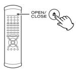
Pressing OPEN/CLOSE opens the tray if it is closed, and closes it if it is open. When the tray is opened during playback, it may take a few seconds before the disc is "unloaded" and the tray opens.
